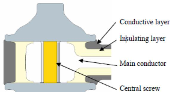
All the external surfaces of the installed interconnector system are screened and connected to the earth. The electrical field is totally included and fixed in the insulating layer without affecting the surface of the interconnector, avoiding any superficial electrical aging.
