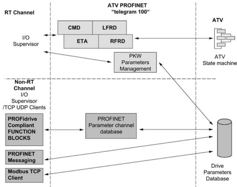
The native mode of the PROFINET VW3A3627 is used when telegram 100 is used.
