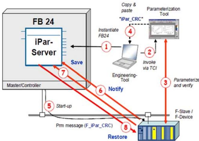
Per upload request, the function block reads the data record with the iParameter out of the drive, creates a data block, and stores the data record therein.
