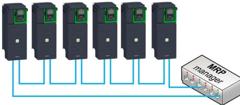
The ring topology can only be used with a media redundancy protocol (MRP) capable managed device. The bus watchdog shall be increased when using MRP function in order to avoid triggering untimely **[Fieldbus Com Interrupt] (L n F)**.
