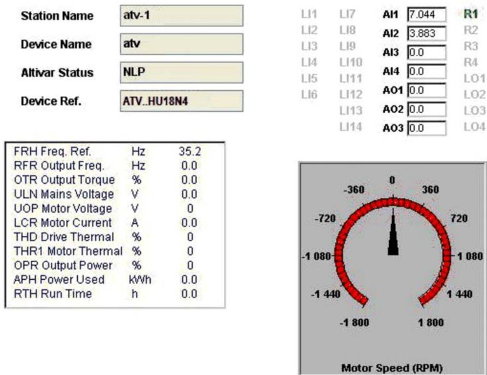
The state displayed in the **Altivar Status** field corresponds to the display on the graphic display terminal. A delay may be noticed between the displays on the Web server and the display terminal. This delay depends on the performance of the computer used to display the pages using a web browser and the communication system performance.
