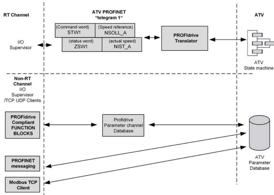
The following section describes how the VW3A3627 is operated when configured in PROFIdrive mode (telegram 1).
