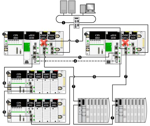
The (red)  $\boldsymbol{X}$  indicates that the BMENOC0301 module is isolated from the Ethernet backplane:
