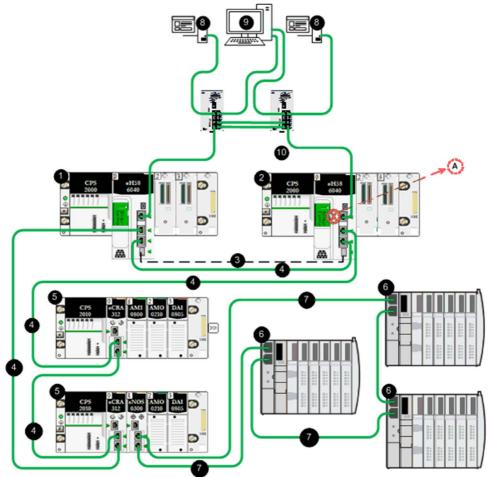
A In this topology, where SCADA is connected to the Hot Standby system via the primary CPU service port and the standby CPU service port, confirm that you select the **Automatic blocking of service port on Standby CPU** check box in the **ServicePort** configuration tab to help avoid network communication loss (formed by cables 4 and 10).
