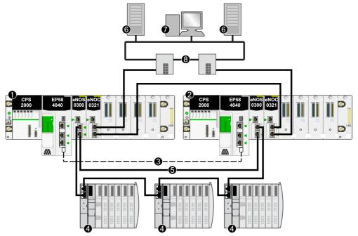
The following example presents a Hot Standby system with a control network communicating with a DIO ring:
