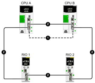
1 Hot Standby fiber optic link between CPU A and CPU B
