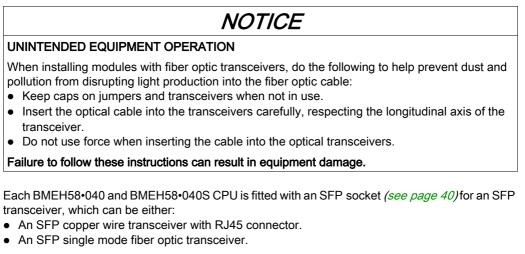
Your choice of connector determines the maximum distance of the Hot Standby physical link.
