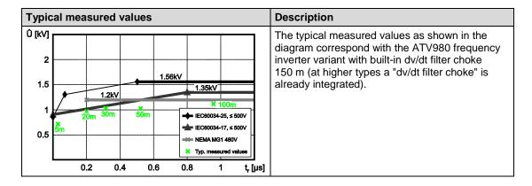
Motors according IEC 60034-25 as well as motors according NEMA MG1 are dimensioned for operation with frequency inverters and thus they are well qualified for drives with ATV980 frequency inverters.
