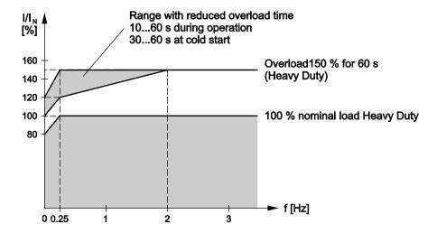
**NOTE:** If the frequency inverter is operated with output frequencies < 2 Hz the overload time at high overload up to 150 % is lower than 60 s. This restriction needs to be observed only for drives which continuously operate around 0 Hz and require overloads up to 150 %.
