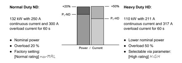
The factory setting of the parameter [Dual Rating] d r k is "Normal Duty". When the product is reset to the factory settings, this parameter is also reset to "Normal Duty".
