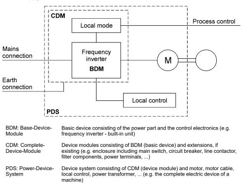
The differentiation in respect of the sales method and the range of use is essential for the handling of frequency inverters.
