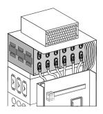
The use of the customization dv/dt filter choke 300 m has significant advantages concerning the operation of the drive:
