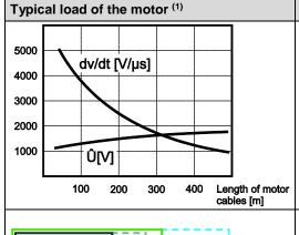
Load of the motor with overvoltage and slew rate when using conventional frequency inverters without integrated dv/dt filter chokes.
