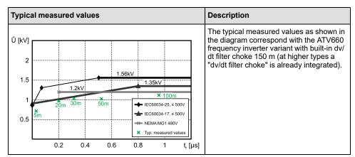
Motors according IEC 60034-25 as well as motors according NEMA MG1 are dimensioned for operation with frequency inverters and thus they are well qualified for drives with ATV660 frequency inverters.
