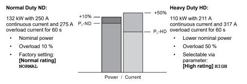
The factory setting of the parameter **[Dual rating]** DRT is "Normal Duty". When the product is reset to the factory settings, this parameter is also reset to "Normal Duty".
