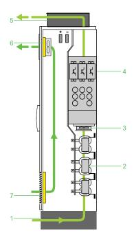
In case of increased protection degree IP54 with separate air channel the cooling air inflow for the power part takes place through the floor and the air outlet through the enclosure roof.
