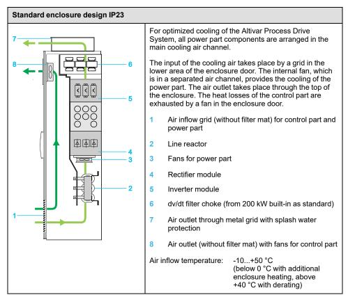
**NOTE:** For details about the increased protection degree IP54 see chapter Increased Protection Degree IP54, page 124.
