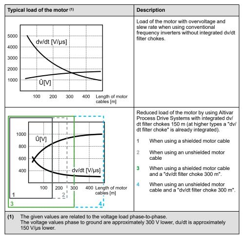
The motor standards for IEC and NEMA specify limits for the permitted load regarding slew rate and voltage peaks
