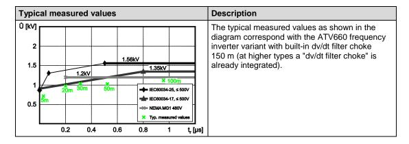
Motors according IEC 60034-25 as well as motors according NEMA MG1 are dimensioned for operation with frequency inverters and thus they are well qualified for drives with ATV660 frequency inverters.
