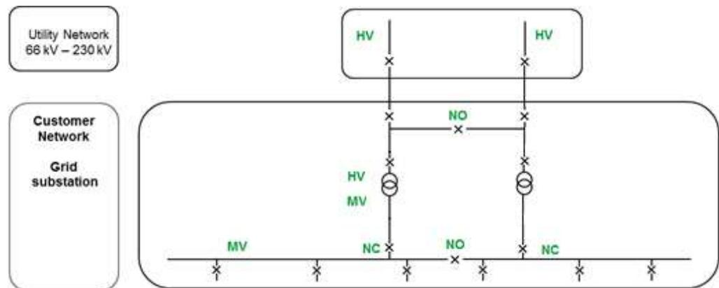
Both transformers are designed to take the full load. Under normal conditions the substation operates with the MV bus section circuit-breaker normally open (NO) and the transformer incomer circuit breaker normally closed (NC) so that the site load is equally shared between the two HV/MV transformers.
