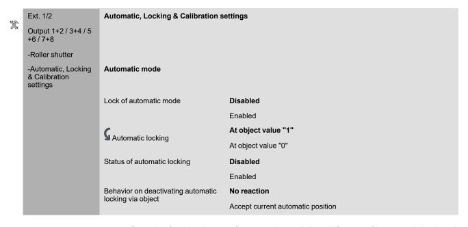
Once the function "Lock of automatic mode" and "Status of automatic locking" has been enabled, new group objects are available for the channel.
