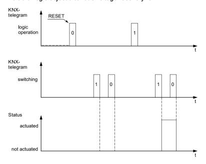
The parameter setting causes the "logic object" to be set to the value "0". After a RESET, the actuator does not switch the output until a "1" telegram has been received on the "logic object".
