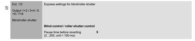
If the channel for a drive that is currently in motion receives a motion command in the opposite direction, it first turns off both output relays for this channel. Before turning on the relay for the new direction of motion, it waits for the set **Pause time before reverting**.
