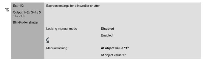
Depending on the setting, manual operation is disabled or enabled when a new telegram value is received:
