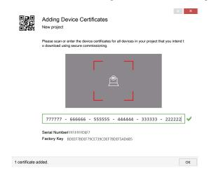
**NOTE:** The certificate consists of the serial number and the security key FDSK (Factory Default Setup Key). The FDSK is only used for initial commissioning and is replaced by the ETS during the first download. This prevents unauthorized persons from gaining access to the installation despite knowing the FDSK.
