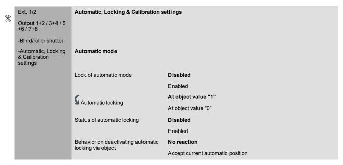
Once the function "Lock of automatic mode" and "Status of automatic locking" has been enabled, new group objects are available for the channel.
