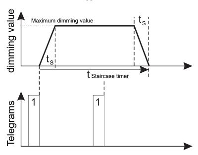
However, if the staircase lighting time is not retriggerable, the output will switch off/dim at exactly the moment the time elapses. If the **Manual Switching off** function is activated, the staircase lighting time can be terminated prematurely with a "0" telegram.
