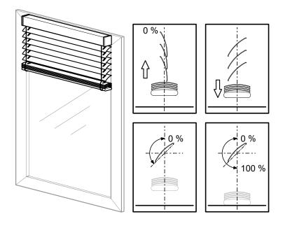
The parameter **Slat position after movement in %** allows you to define the behavior of the slats after a movement for the channel.
