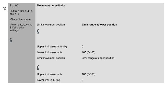
The movement range limitation function is often selected in summer when solar radiation is strong, so that it does not heat up rooms or dazzle people. The drive can no longer be moved manually all the way up, but in the event of a storm the weather alarm will move the blind to the safe position.
