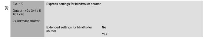
To activate the extended settings for blind/roller shutter, you must enable them here.
