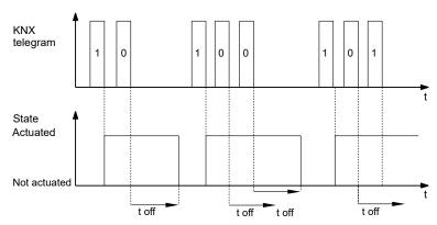
Moreover, for the off-delay, you can also select **Retriggerable and adding**. The delay time is added when the same telegram value is received, e.g. using a separate button. You can define the maximum number of additions.
