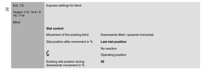
You can use the parameter **Existing slat position during downwards movement in %** to set the opening angle for the operating position.
