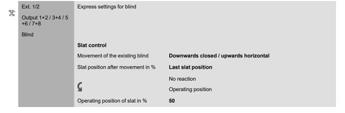
The preset value of 50% corresponds to a slat opening angle of about 45°. Since this position is set on a time-controlled basis, please refer also to the section Slat Rotation Time, page 116.
