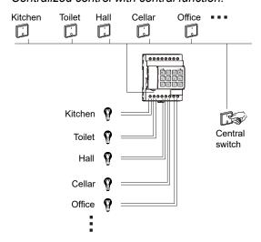
Dimming, switching, blind and roller shutter each have a separate **central object** with a corresponding **central object**. In order to use the **central function** for the individual dimming, switch/blind/roller shutter channels, you must first enable the global function on the **General settings** tab.
