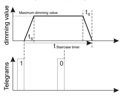
A telegram with the object value **0** has no effect. The set **staircase light time** continues to run normally until the end.
