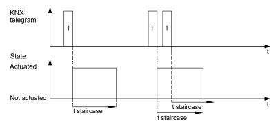
However, if the staircase lighting time is not retriggerable, the relay will switch off at exactly the moment the time elapses.
