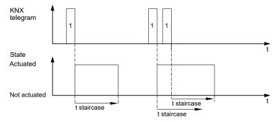
Once a new telegram with the object value "1" has been received, the staircase lighting time is restarted.
