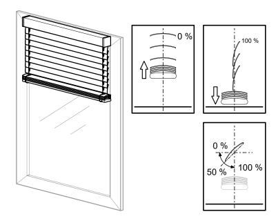
The parameter **Slat position after movement in %** allows you to define the behavior of the slats after a movement for the channel. If you set the parameter to **Operating position**, you can set an opening angle to be adopted by the slats after every downward movement.
