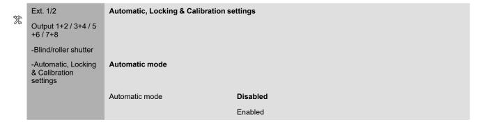
In order to use the **automatic mode**, you must first activate the function in the ETS. Once **automatic mode** has been enabled, new group objects are available for the channel.
