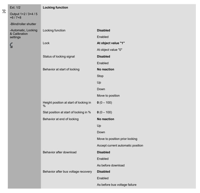
Once the **Locking function** and **Status of locking signal** have been enabled, new group objects are available for the channel.
