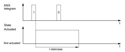
A telegram with the object value **0** has no effect. The set staircase light time continues to run normally until the end.
