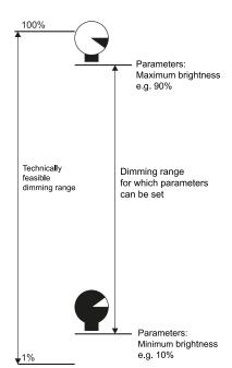
The **dimming range** can be limited further using the software application. This limit can be set individually for each output channel.
