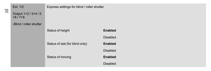
Each blind channel can provide different status responses, depending on how it is enabled. The status response group objects are available and can be disabled.
