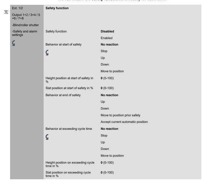
The safety function is activated if the **safety object** receives a telegram with the object value that you defined with the parameter **Device safety** (). You can define the reaction using the parameter **Behavior at start of safety**.
