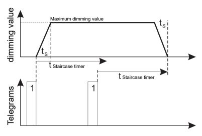
Once a new telegram with the object value "1" has been received, the staircase lighting time is restarted.
