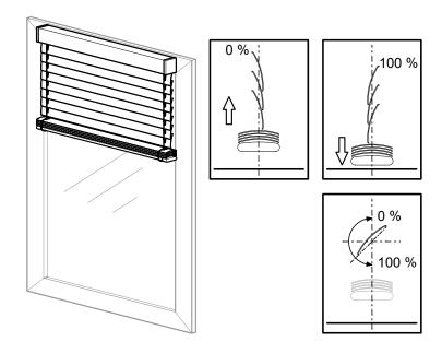
The parameter **Slat position after movement in %** allows you to define the behavior of the slats after a movement for the channel. If you set the parameter to **Operating position**, you can set an opening angle to be adopted by the slats after every downward movement.
