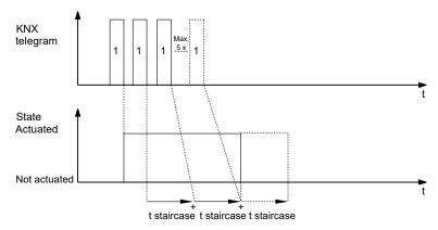
Once one or more new telegrams with the object value "1" have been received, the staircase lighting time is added to the previous staircase lighting time. The number of additions can be set. You can parameterize a maximum of 5 additions of the staircase lighting time.
