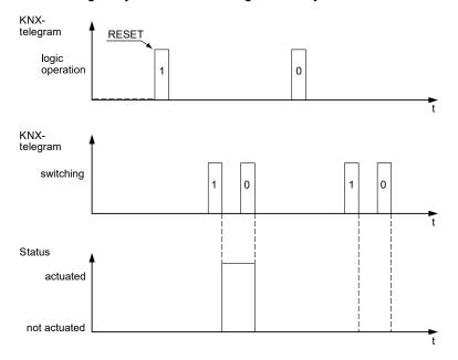
The logic object is preset with the value "1" after a RESET (bus voltage recovery and download). This enables switching to be carried out as usual using the switch object. The power-on lock is not active until a "0" telegram has been received via the logic object.
