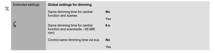
The group object appears after the enabling **Control same dimming time via bus**.
