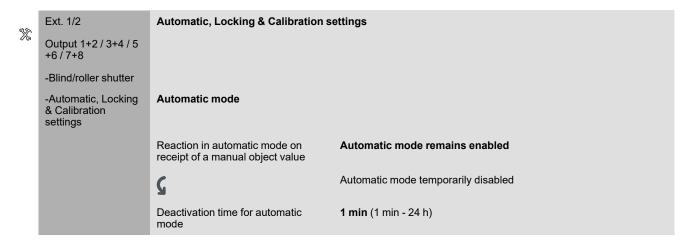
Permanent deactivation of the automatic function can only be canceled by a telegram terminating automatic locking via the automatic locking object. The action you set in the parameter "Behavior on deactivating automatic locking via object" will be executed.
