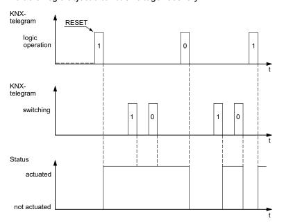
The logic object is preset to the value "1" after a RESET. The actuator will switch on the output immediately. The OR logic function is only reset by a "0" telegram on the logic object.
