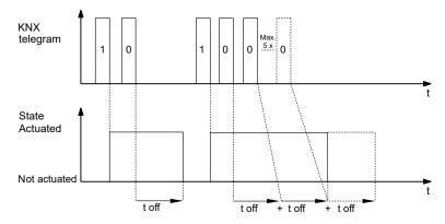
In the case of not retriggerable delays, by contrast, the relay will switch off at exactly the moment the time elapses.
