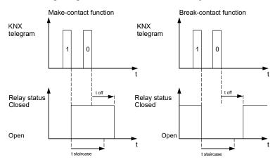
For staircase lighting time functions with **manual switching off** and warnings activated, the staircase lighting time function is immediately deactivated with a warning when an "Off" telegram is received. The off-delay elapses. No warning is generated.
