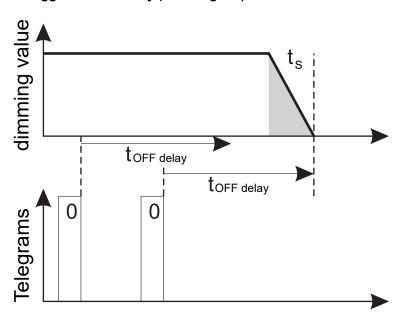
Moreover, for the off-delay, you can also select **Retriggerable and adding**. The delay time is added when the same telegram value is received, e.g., using a separate button. You can define the maximum number of additions.
