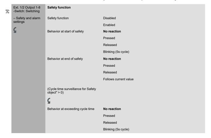
The safety function is activated if the **safety object** receives a telegram with the object value that you defined with the parameter **Device safety** (). The reaction is defined by the parameter **Behavior at start of safety**.
