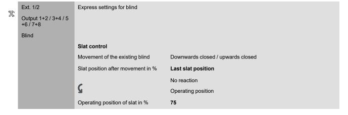
The preset value of 75% corresponds to a slat opening angle of about 45°. Since this position is set on a time-controlled basis, please refer also to the section Slat Rotation Time, page 116.
