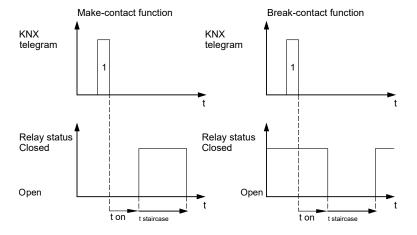
The result of combining a staircase lighting time function with an off-delay depends on how you have defined the **staircase lighting time** function:
