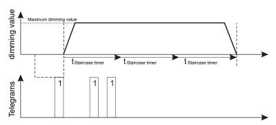
Once one or more new telegrams with the object value "1" have been received, the staircase lighting time is added to the previous staircase lighting time. The number of additions can be set. You can parametrize a maximum of 5 additions of the staircase lighting time.
