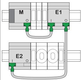
An extension cannot be put into operation if the order of the devices does not correspond to your programming in the ETS.
