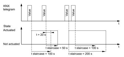
Once a new telegram has been received, the staircase lighting time is restarted with the higher value.
