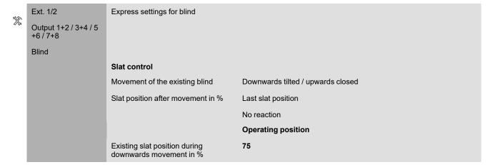
You can use the parameter **Existing slat position during downwards movement in %** to set the opening angle for the operating position.
