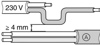
The diagram shows a 230V supply cable with two conductors and a ground wire. Below it, a KNX line with two conductors is shown. A dimension line indicates a minimum distance of 4 mm between the conductors of the 230V cable and the conductors of the KNX line.
