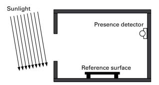
Optimal light conditions for actual value correction. Measurement results at the installation site or at the reference area are affected equally by natural light.
