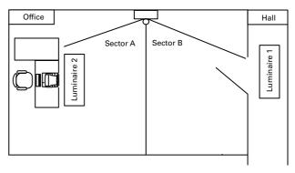
Luminaire 1 should only switch on when there is a movement in the hall.
