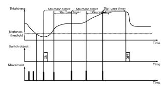
Where this differs from the presence detector is that the movement detector changes to non-brightnessdependent mode once the start of movement action (sending an ON telegram) has been carried out. Here freshly detected movements can retrigger the staircase timer. Unlike the presence detector, the movement detector cannot process the brightness jump and there is not even any setting of a hysteresis.
