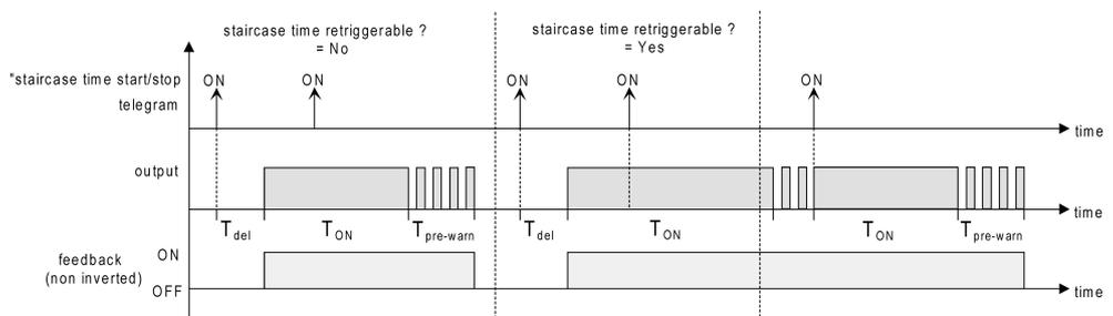
Image 24: Switch-on behaviour of the staircase function
