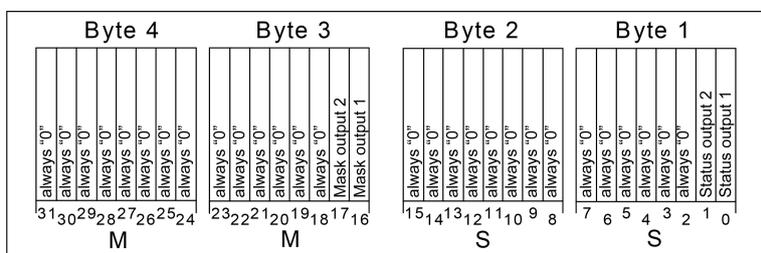
Image 23: Object structure of the collective feedback
