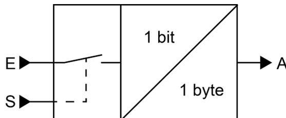
Image 46: Converter (1 bit -> 1 byte)
