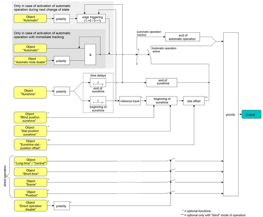
Image 17: Function diagram illustrating the extended sun protection
