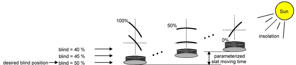
Image 10: Example of slat positioning affecting the position of the Venetian blind (typical of slat type 1; analogous reaction for type 2)
