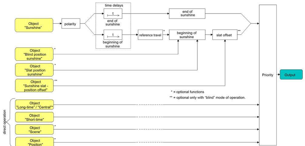
Image 15: Function diagram illustrating the simple sun protection
