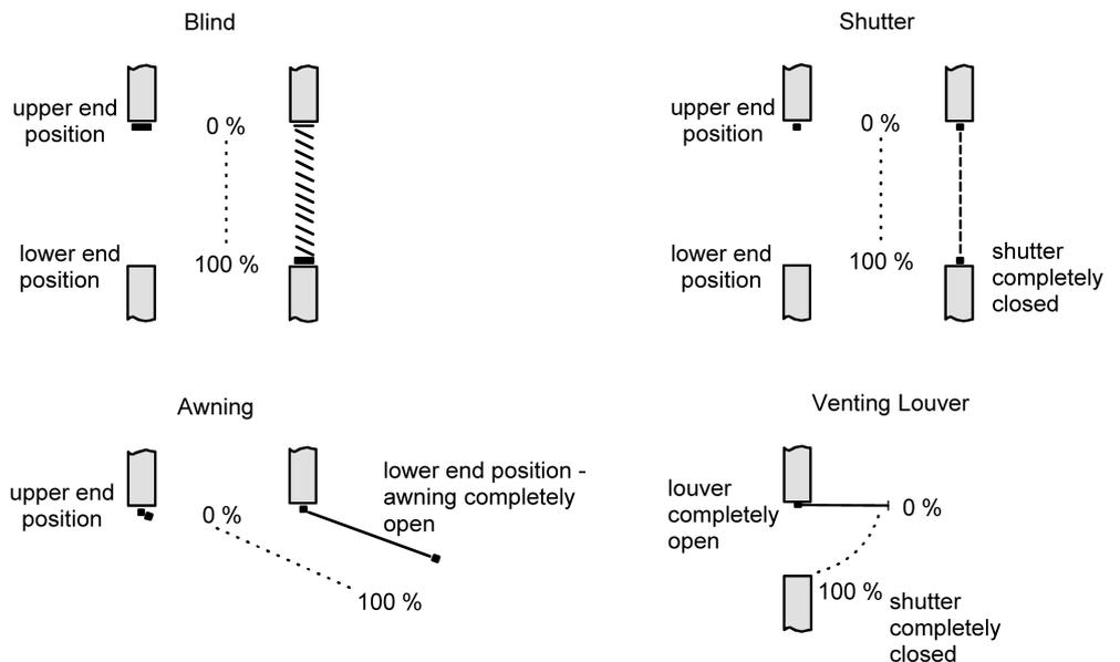
Image 9: Positions defined as a function of the type of movement
