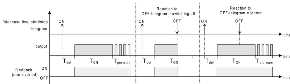
Image 25: Switch-off behaviour of the staircase function
