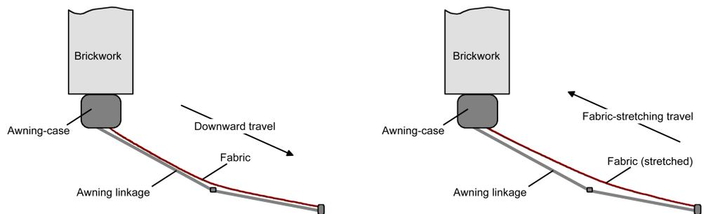
Image 21: Fabric stretching in an awning
