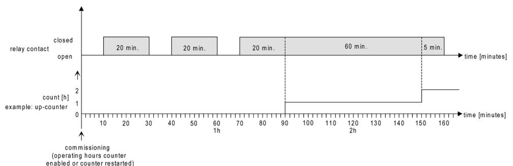
Image 29: Function of the operating hours counter (using the example of counted hours)
