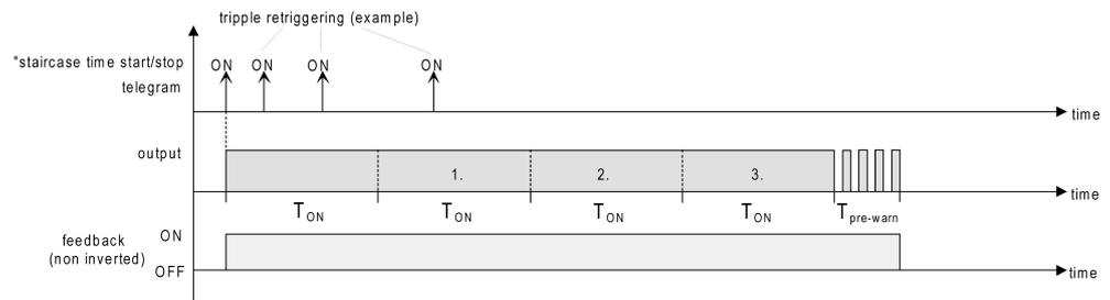
Image 27: Time extension of the staircase function
