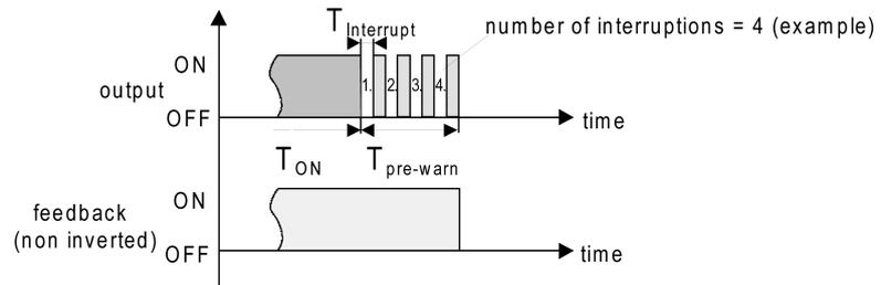
Image 26: The pre-warning function of the staircase function (example)
