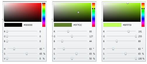
Image 23: Examples of brightness adjustment using the colour picker of the ETS Examples of HSV-RGB conversion:
