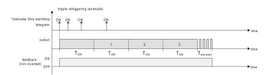
Image 9: Time extension of the staircase function
