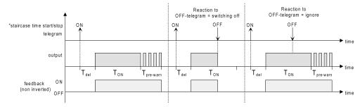
Image 7: Switch-off behaviour of the staircase function
