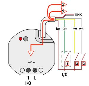
Image 12: Functionality of the input 1 when controlling the internal
