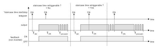
Image 6: Switch-on behaviour of the staircase function
