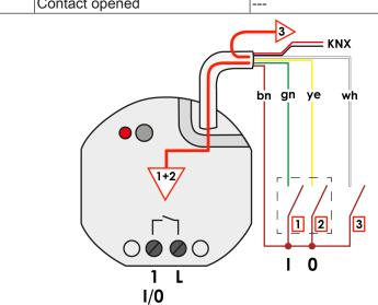
Image 13: Functionality of the inputs when controlling the internal Switching output as dual-area operation
