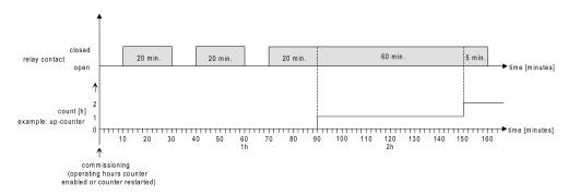
Image 11: Function of the operating hours counter (using the example of counted hours)
