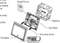
Insert a screwdriver into the clip lock, and twist the screwdriver to remove the faceplate.
