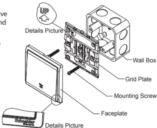
Insert a screwdriver into the clip lock, and twist the screwdriver to remove the faceplate.
