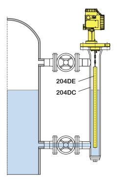
Transmitter and Shut-off device Displacer 204DE in Displacer Chamber 204DC
