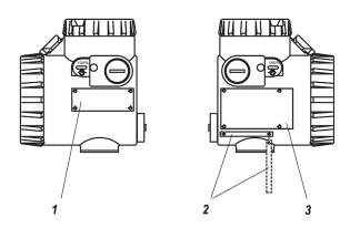
The transmitter is identified with three labels. The transmitter nameplate **3.1** shows the Model Code of the transmitter, which clearly describes the device. The certificate data and the serial No. are entered on the amplifier nameplate **3.3**. The TAG No. label **3.2** with the Tag No. is located underneath (optional). Data about the permissible static pressure and the displacer are documented on the data label **3.4** on the process connection flange.
