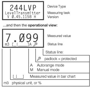
The operational view is the display in normal operation.
