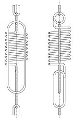
It is hooked onto the suspension chain of the displacer in place of 7 chain links (105 mm). This spring is specially matched to the resonance frequency of the displacer and is made of stainless steel (material 1.4310, max. operating temperature 250°C).
