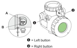
After shifting the key protection cap **A**, insert screw driver or pin ( $\emptyset$  < 3 mm) into hole **B** and press down to the second pressure point.
