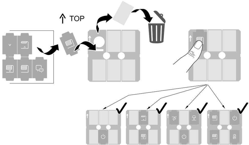
**i** If the symbol is not entirely straight: Detach the symbol and then stick it on again. The procedure can be run through repeatedly.
