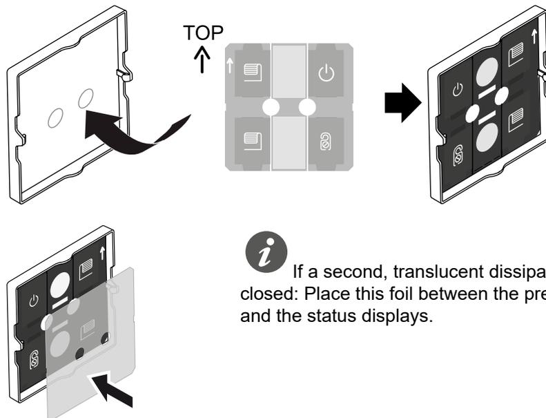
**i** If a second, translucent dissipative foil is enclosed: Place this foil between the prefabricated foil and the status displays.
