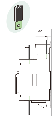
Busbar to Base Plate
