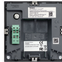
Connection with FDM121 display unit.
