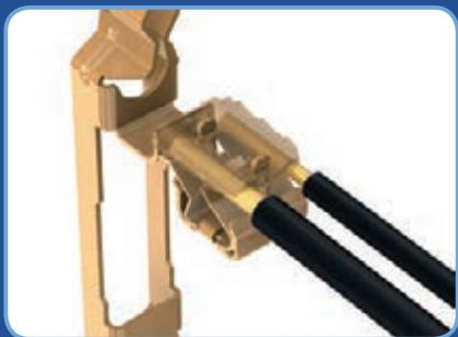
Screwless internal cable clipping system: The individual clamping system guarantees perfect and safe cable connection even with different diameters.
