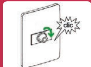
**Product activation:** 300\* rotary setting for dimmers and fan speed control (on/off integrated)
