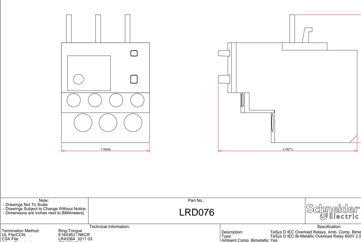
CSA File: Meets Standard: IEC 60947-1 CE: RoHS: Weight: Power Wire Size : Control Wire Size: Yes Yes 0.12 lb (0.27 kg) Lug Size 0.32 in (8mm) Lug Size 0.32 in (8mm) 15 lb-in (1.7 Nm) Power Terminal Torque: Control Terminal Torque: 15 lb-in (1.7 Nm) Mtg. Directly to Contactor: Yes Mtg. Separate from Contactor: LAD7B10
