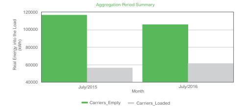
Ratio of energy consumed when carriers were running empty vs. loaded was improved significantly, increasing throughput .
