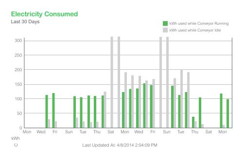
Consumption vs. Process Energy Usage: Energy consumed during idle conveyor time was unexpectedly high, uncovering a process inefficiency .
