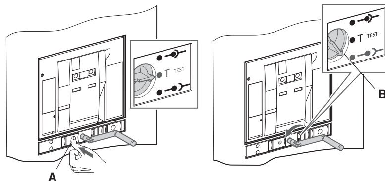
Figure 75 – Rack Circuit Breaker to Disconnected Position
