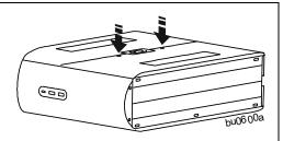
Press the tabs downwards and pull the battery door away from the unit to access the battery modules.
