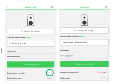
Current version appears : - in grey if « up to date » or if eSetup has never been open with data connection - in red if a new version has been detected by eSetup on the Schneider Cloud
