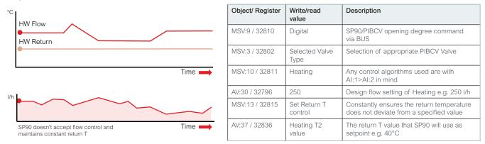
Note: SP90 defaults to select metric units of measurement, I/h, 0°C, Kw
