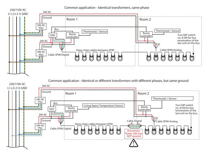
Wires that ends in an "X" must be properly terminated.
