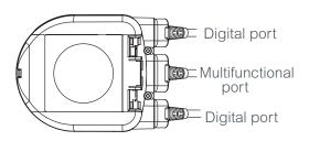
The length of the cables influence on the communication speed. Longer cable lengths should result in lower baud rates. The total maximum cable length allowed per network is 1200m. Use a minimum 20 cm distance between 110V/230V/400V power line cables and bus cables.
