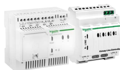
Exiway Smart Control - Control Unit 128 to control up to 128 Dicube devices consisting of the control unit and a Line Controller module (2 lines of 64 devices)
