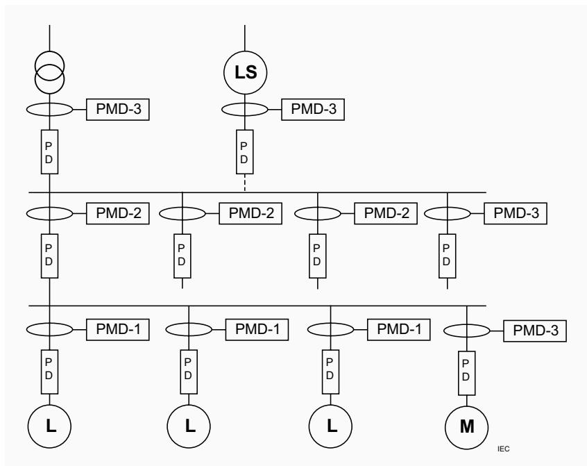
**Figure 2:** Example of measurement equipment selection in an installation (Paragraph 8.3.1.3 of the standard).
