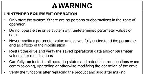
Verify the functions after replacing the product and also after making modifications to the parameter values and/or other operational data.
