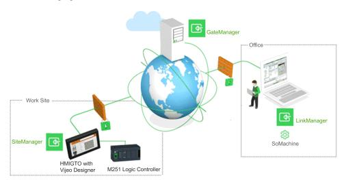
**NOTE:** The HMIGTO appliance and the M251 Logic Controller must be on the same network at the work site. Modify IP addresses that appear in this guide to those used on your network.
