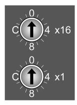
**NOTE:** Any modification of the rotary switch position is taken into account only after the next power cycle.
