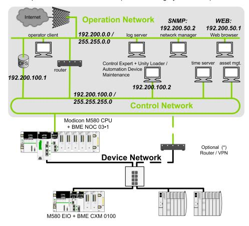
(\*) Some services require access to the device network (for example: firmware update, at source time stamping). In such cases, an optional router/VPN helps secure the access control.
