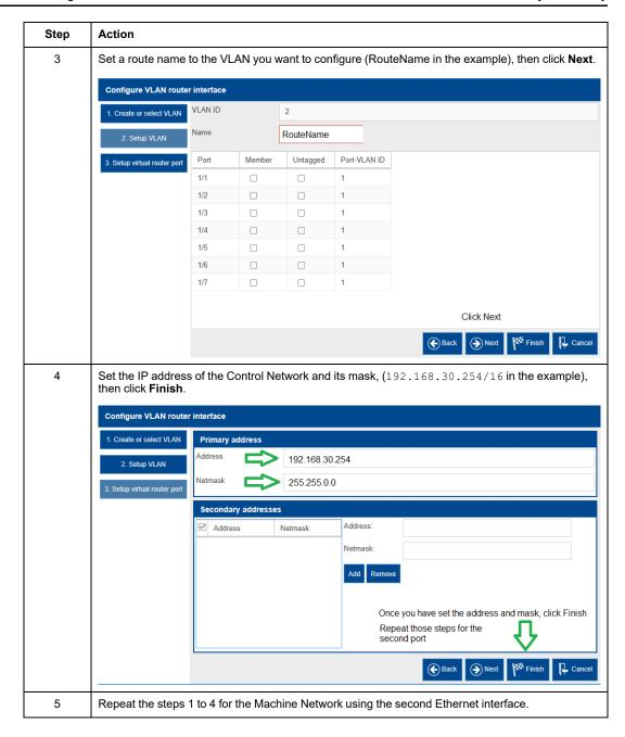
In the following example we have set the control network gateway interface of the firewall to 192.168.30.254/16 on the physical port n°1 and machine network to 139.160.235.254/16 on the physical port n°2.
