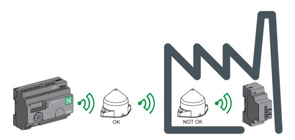
**NOTE:** The antenna should be placed before the obstacle. The signal will be amplified before the obstacle to enable to go through it.
