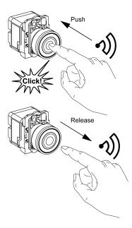
The radio message is sent when the button is pressed, signaled by a click.
