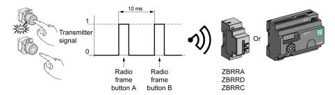
ZBRT1 is used for applications where single pulse is required (for example, remote start of machine and reset after machine fault detection).
