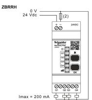
(2): 500 mA fuse from supplier Bussman® reference GMA-500 mA, 250 V 0.5 A fast-blow.
