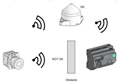
You can also use the relay antenna to amplify the signal before an obstacle that cannot be bypassed, such as a factory building as shown in the following figure:
