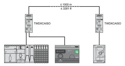
For distances longer than 20 m (65.62 ft), verify that the other devices connected to the bus are isolated. If other devices are not isolated, use the TWDXCAISO module.
