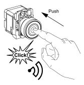
The radio message is sent when the button is pressed, signaled by a click. If the button is held down, the message is not transmitted continuously. The message is not sent when the button is released.
