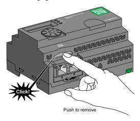
Push to remove the SD card from the SD card slot on Harmony Hub.
