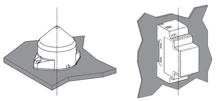
The antenna and the receiver are installed following their vertical axis.
