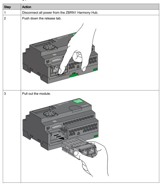
ZBRCETH offers one Ethernet communication port equipped with two RJ45 plugs. It enables daisy chain wiring between devices without using a switch.
