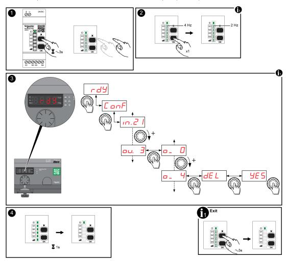
**NOTE:** The Q1...Q4 outputs are active during 1 s after the teaching procedure.
