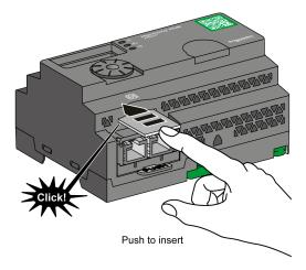
Push to insert the SD card into the SD card slot on Harmony Hub. Make sure that the SD card is inserted properly.
