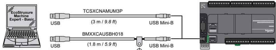
The following illustration shows the USB connection to a PC on a TM221M Logic Controller:
