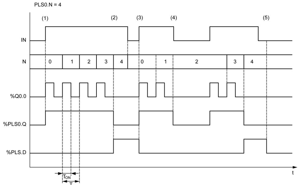
(1) *IN* input is set to 1, the pulse signal is generated at the dedicated output ( $\%Q0.0$ ) so  $\%PLSi.Q$  is set to 1
