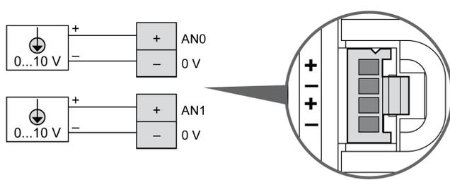
The (-) poles are connected internally.
