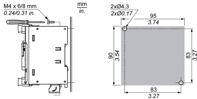
The following diagram shows the mounting hole layout for TM221C Logic Controller with 24 I/O channels:
