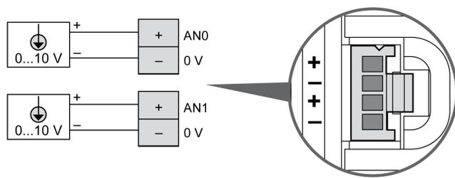
The (-) poles are connected internally.
