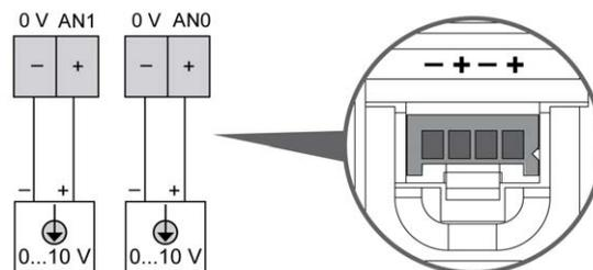
The (-) poles are connected internally.
