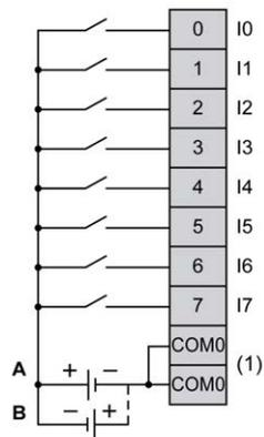
(1) The COM0 terminals are connected internally.
