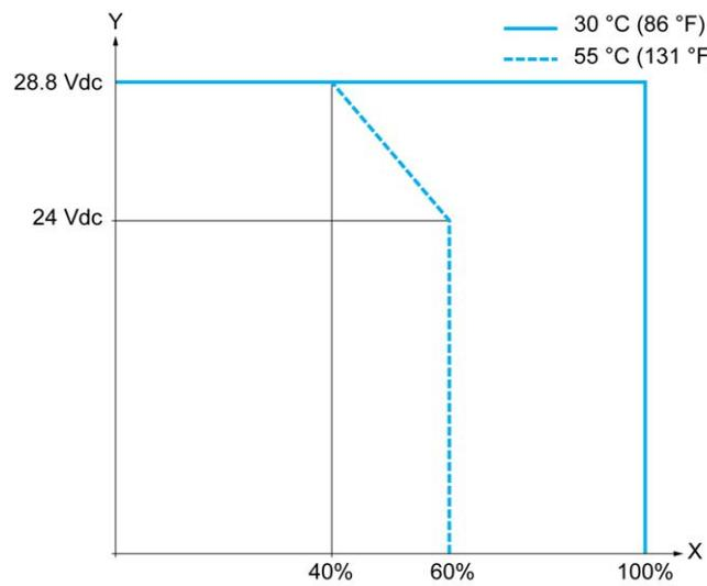
**X** Input simultaneous ON ratio
