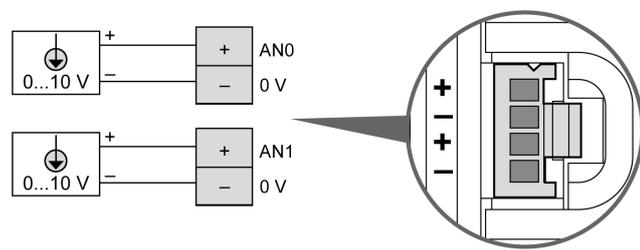
The (-) poles are connected internally.
