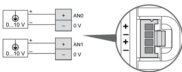
The (-) poles are connected internally.
