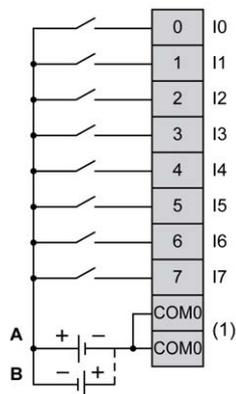
**(1)** The COM0 terminals are connected internally.
