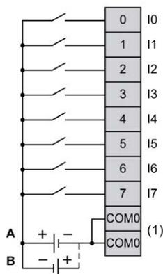
(1) The COM0 terminals are connected internally.
