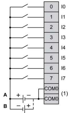
(1) The COM0 terminals are connected internally.
