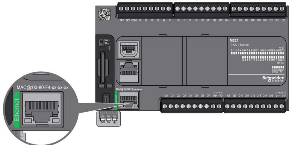
The following figure presents the location of the Ethernet port on the TM221M Logic Controller:
