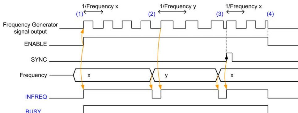
(1) The *ENABLE* input is set to 1. The frequency generator signal is generated at the dedicated output. The *INFREQ* output is set to 1. The *BUSY* output is set to 1.
