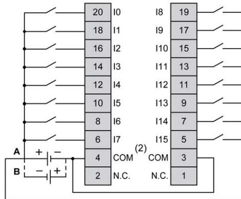
(1) The COM terminals are **not** connected internally.
