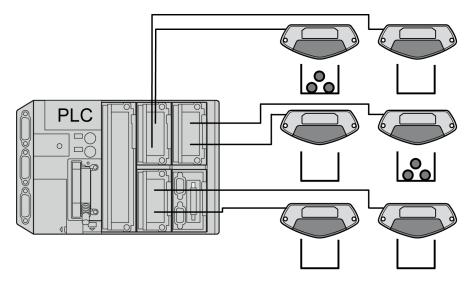
In this mode, each Picking Sensor XUPK1 is wired to the PLC by direct point-to-point connection.
