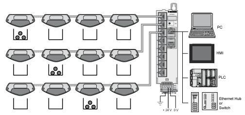
You can connect to a XUPH Communication Box up to 64 Picking Sensors XUPK2, maximum 14 per daisy-chain.
