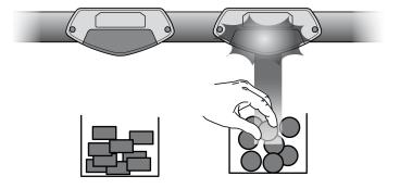
Depending of the user mode chosen, the system can manage the lightning of LEDs: right side or left side, continuous light or flashing, for a time period, with delays or not.
