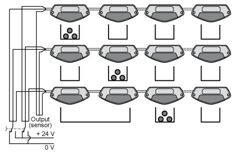
On the Picking Sensors network, you can connect up to 64 Picking Sensors XUPK1, maximum 14 per daisy-chain.
