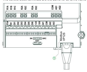
1 Modbus VP12S: This is the standard Modbus serial link marking. VP•S means connector with power supply, where 12 stands for the 12 Vdc supply voltage.
