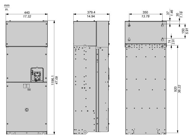
**NOTE:** Lower Conduit Box part sold separately. This part enables wall mounting of the product. It provides IP21 protection degree on the bottom side.
