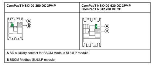
The SD auxiliary contact for BSCM Modbus SL/ULP module cannot be installed at the same time as the SD contact.
