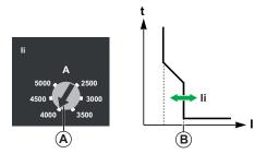
The following table shows the values of the pick-up li (in amperes) for magnetic protection (values indicated on the dial), relative to the position of the li dial:
