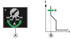
The following table shows the values of the pick-up Ir (in amperes) for thermal protection (values indicated on the dial) with respect to every trip unit rating, relative to the position of the dial Ir.
