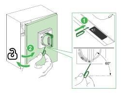
The rotary handle is delivered with the door lock activated. To deactivate the lock, consult the instruction sheets:
