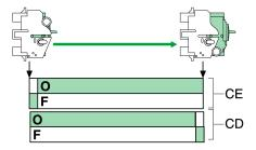
CE Connected position carriage switch
