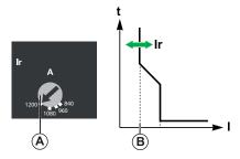
The following table shows the values of the pick-up Ir (in amperes) for thermal protection (values indicated on the dial) with respect to every trip unit rating, relative to the position of the dial Ir.
