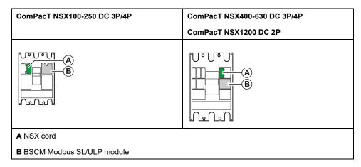
The NSX cord cannot be installed at the same time as the SD auxiliary contact.
