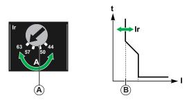
The following table shows the values of the pick-up Ir (in amperes) for thermal protection (values indicated on the dial) with respect to every trip unit rating, relative to the position of the dial Ir.
