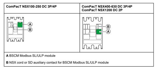
The BSCM Modbus SL/ULP module cannot be installed at the same time as an OF contact or the SDE contact.
