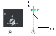
The following table shows the values of the pick-up Ir (in amperes) for thermal protection (values indicated on the dial) with respect to every trip unit rating, relative to the position of the dial Ir.
