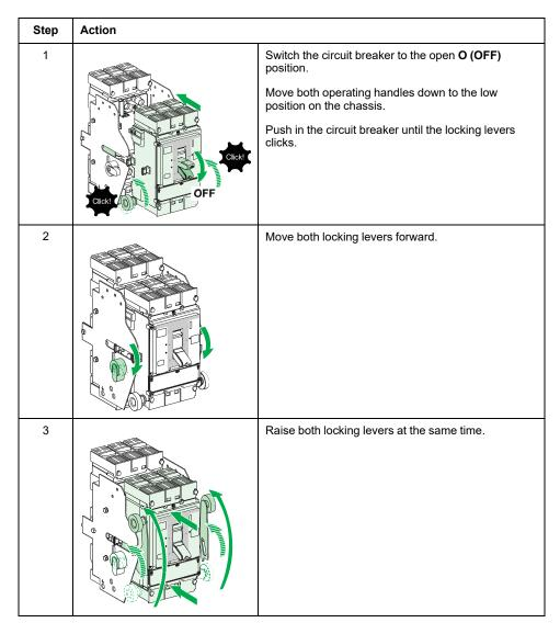
**NOTE:** Open the circuit breaker before connecting it. If the circuit breaker is in the closed **I (ON)** position when connecting, a safety mechanism ensures that the poles open automatically by tripping the circuit breaker before the pins connect.
