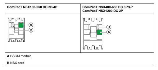
The BSCM module cannot be installed at the same time as an OF contact or the SDE contact.
