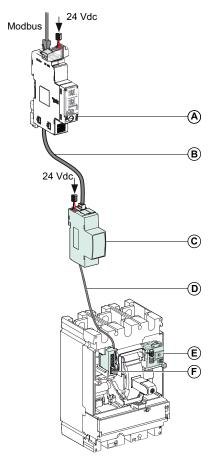
A IFM Modbus SL communication interface for one circuit breaker
