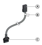
A RJ45 plug to Modbus SL hub
