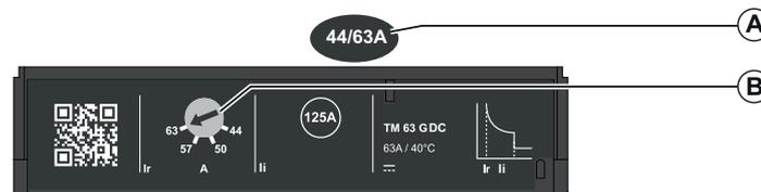
**A** Setting range for the TM-G thermal-magnetic trip unit
