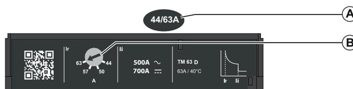
**A** Setting range for TM-D thermal-magnetic 3P/4P trip unit
