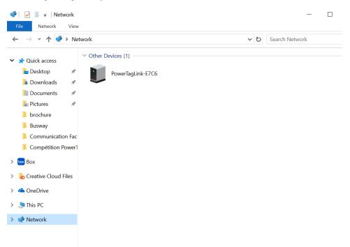
If the PowerTag Link gateway IPV4 is in DHCP mode, the PC must also be in DHCP mode. If PowerTag Link gateway uses a static IP, the PC must also use a static IP in the same network (same Subnet mask).
