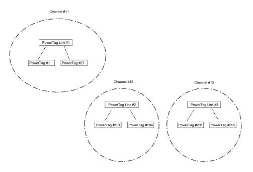
Both PowerTag Link gateway (A9XMWD20) and PowerTag Link HD gateway (A9XMWD100) must use its own wireless channel that is different from the wireless channels used by the other gateways, if applicable. For any installation with multiple gateways, refer to <u>DOCA0194EN</u> PowerTag System - Design and Commissioning Guide or contact Schneider Electric customer support.
