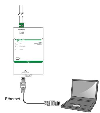
PowerTag Link gateway has an embedded web server. A web server is used to set Ethernet parameters or to display wireless devices configured with EcoStruxure Power Commission software or with webpages.
