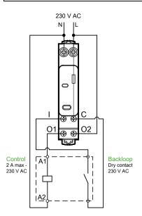
**NOTE:** It is not possible to use the input of the PowerTag control IO module as an independent input from the control circuit of the output. This input is dependent on the output and used as backloop.
