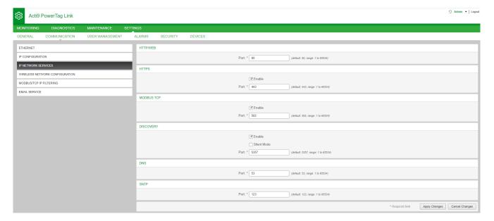
The PowerTag Link gateway supports HTTPS/HTTP, Modbus/TCP, DNS, SNTP, and discovery services.
