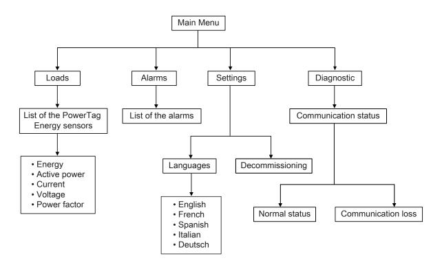
The **Loads** menu displays the list of the PowerTag Energy sensors identified by the **Asset Name** of the PowerTag Energy sensors being configured.
