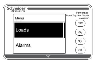
**NOTE:** It takes up to 10 minutes to synchronize the asset name list of the PowerTag Energy sensors and to display in the **Loads** menu.
