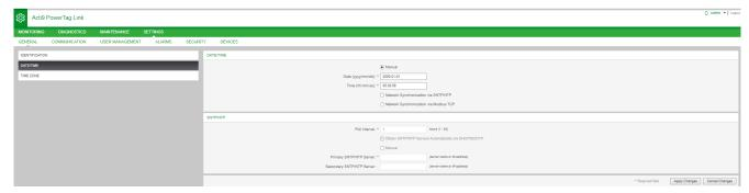
**NOTE:** After the power shut down of any gateway, the gateway will reset to a default value of date and time. The default date and time value is 2000/1/1, 00:00:00.
