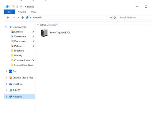
If the PowerTag Link gateway IPV4 is in DHCP mode, the PC must also be in DHCP mode. If PowerTag Link gateway uses a static IP, the PC must also use a static IP in the same network (same Subnet mask).
