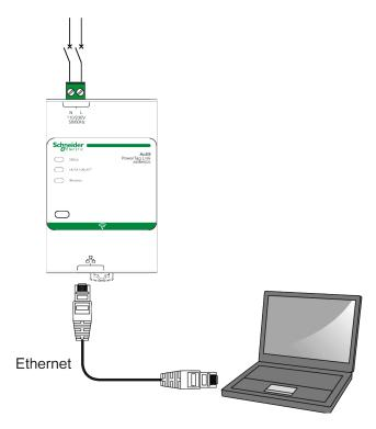
PowerTag Link gateway has an embedded web server. A web server is used to set Ethernet parameters or to display wireless devices configured with EcoStruxure Power Commission software or with webpages.
