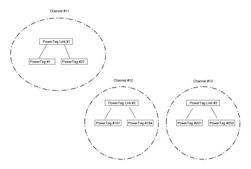
Both PowerTag Link gateway (A9XMWD20) and PowerTag Link HD gateway (A9XMWD100) must use its own wireless channel that is different from the wireless channels used by the other gateways, if applicable. For any installation with multiple gateways, refer to <a href="DOCA0194EN">DOCA0194EN</a> PowerTag System - Design and Commissioning Guide or contact Schneider Electric customer support.
