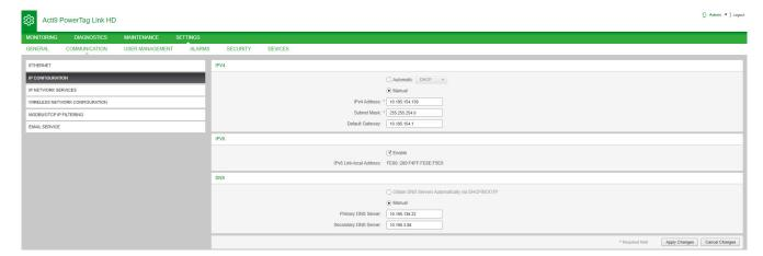
IPv4 parameters can be set either in manual mode or in automatic mode. To configure IPv4 parameter in automatic mode, click **Automatic** and select the type of protocol (DHCP or BOOTP) from the list. The default type is **DHCP** protocol.
