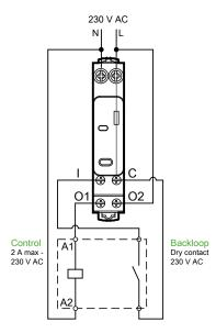
**NOTE:** It is not possible to use the input of the PowerTag control IO module as an independent input from the control circuit of the output. This input is dependent on the output and used as backloop.
