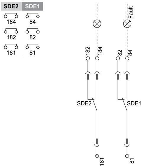
SDE1 fault-trip indication contact and RES remote reset
