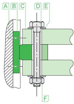
**A** Terminal screw factory-tightened to 13 N•m (MasterPact MTZ1) and 17 N•m (MasterPact MTZ2/MTZ3)
