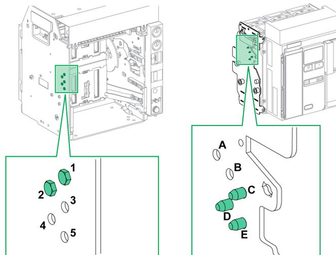
The pin combination selected on the chassis must correspond to the pin combination selected on the device (see following table). For example, the combination 12 on the chassis corresponds to the combination CDE on the device.
