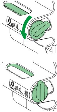
The diagram consists of two parts. The top part shows a close-up of the handle knob with a green arrow indicating a clockwise rotation. The bottom part shows the knob after rotation, with a slot opening on its side. |
