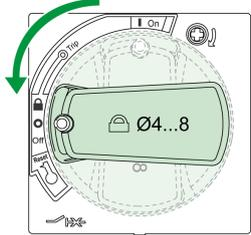
A top-down view of the circuit breaker handle. The handle is a green rectangular shape with a circular lock in the center. It is currently in the 'ON' position, indicated by a green arrow pointing upwards. A green curved arrow above the handle indicates the direction of rotation to the 'OFF' position. The handle has 'I ON' and 'O OFF' markings. A label 'Ø4...8' is visible on the handle.   |
