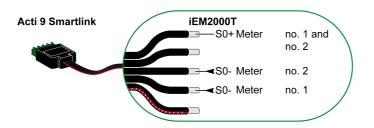
**NOTE:** A single Acti 9 Smartlink channel can take account of 2 meters, 1 meter on input I1 and 1 meter on input I2.
