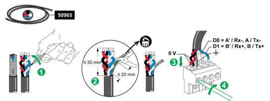
The table below describes the procedure for connecting the Modbus connector:
