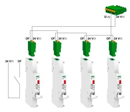
(1) Input I1 (of a channel) on Acti 9 Smartlink or PLC input
