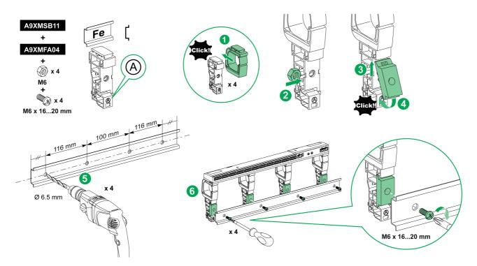
The table below describes the procedure for mounting the Acti 9 Smartlink device on a simple DIN rail:
