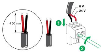
The table below describes the procedure for connecting the power supply connector:
