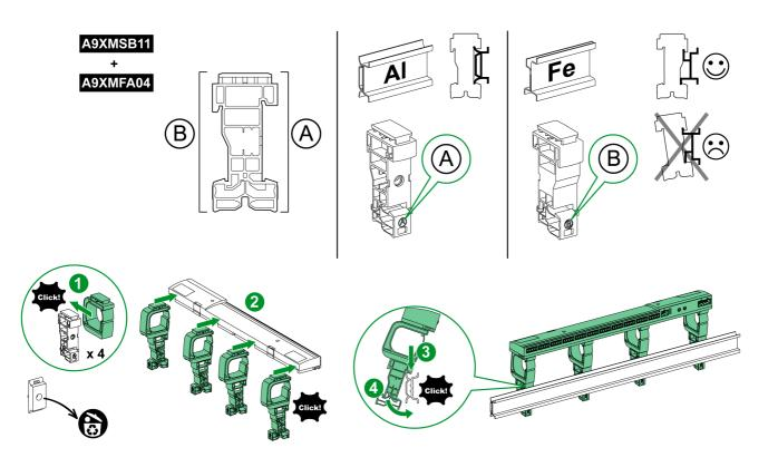
The table below describes the procedure for mounting the Acti 9 Smartlink device on a DIN rail:
