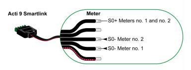
**NOTE:** A single Acti 9 Smartlink channel can take account of 2 meters, 1 meter on input I1 and 1 meter on input I2.
