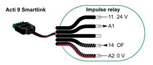
The impulse relay wiring diagram is:
