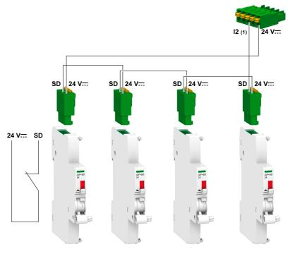
(1) Input I2 (of a channel) on Acti 9 Smartlink or PLC input
