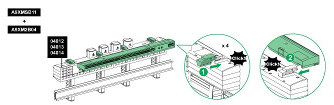
The table below describes the procedure for mounting the Acti 9 Smartlink device on Multiclip 200.
