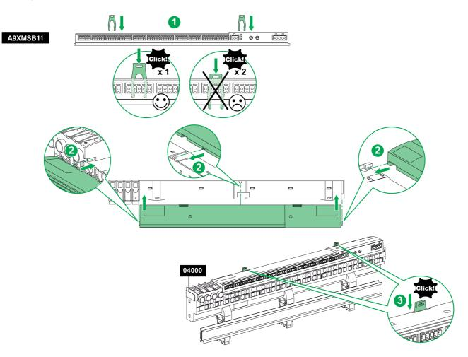
The table below describes the procedure for mounting the Acti 9 Smartlink device on Multiclip 80.
