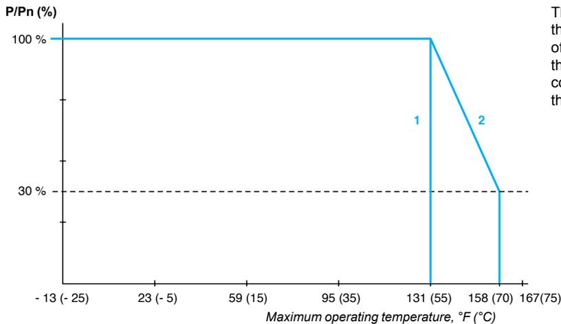
The graph to the left shows the power as a percentage of the nominal power that the power supply can deliver continuously, depending on the ambient temperature.
