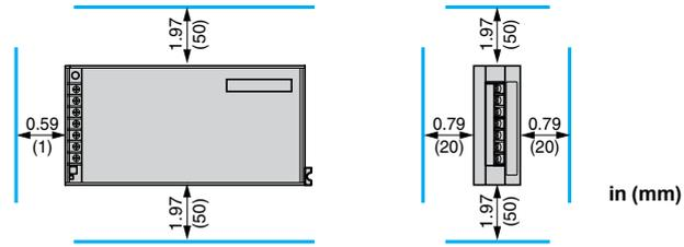
In all cases, there must be adequate convection around the products to help ensure sufficient cooling. There must be a clear space of 1.97 in (50 mm) above and below the power supplies, and of 0.79 in (20 mm) at the sides.
