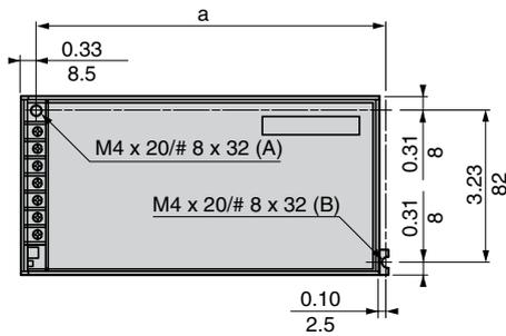
Back-of-cabinet mounting using the ABL1A01 reversible bracket with 3 Ø 4 mm screws
