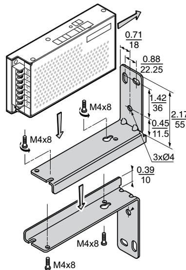
Plate-mounting using the ABL1A02 clip-on plate on a 35 mm DIN rail
