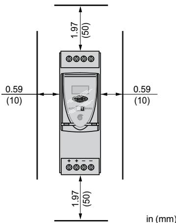
In all cases, there must be adequate convection around the products to assist cooling. There must be sufficient clearance around the Optimum range Phaseo power supplies:
