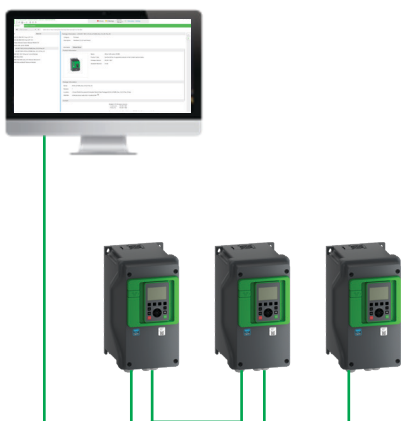
Firmware upload of several ATH600s at the same time through Modbus TCP/Ethernet/IP or Modbus serial using Ecostruxure Automation Device Maintenance
