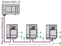
ATV320 Compact + VW3A3600 + module VW3A3608
