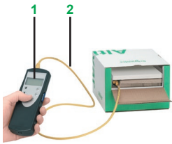
Configuring the drive in its packaging with the Multi-Loader tool VW3A8121+ cordset VW3A8126
