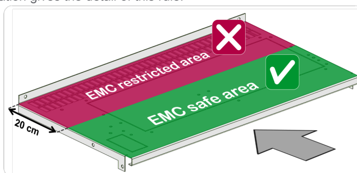
Picture 15: EMC areas identification – Front face
