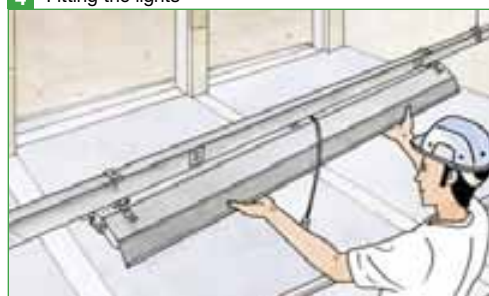
4 Fitting the lights
