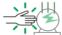
Contact of persons with conductive parts that are accidentally powered as a result of an insulation failure.
