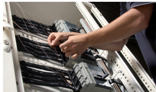
Temperature rise test in laboratory.
